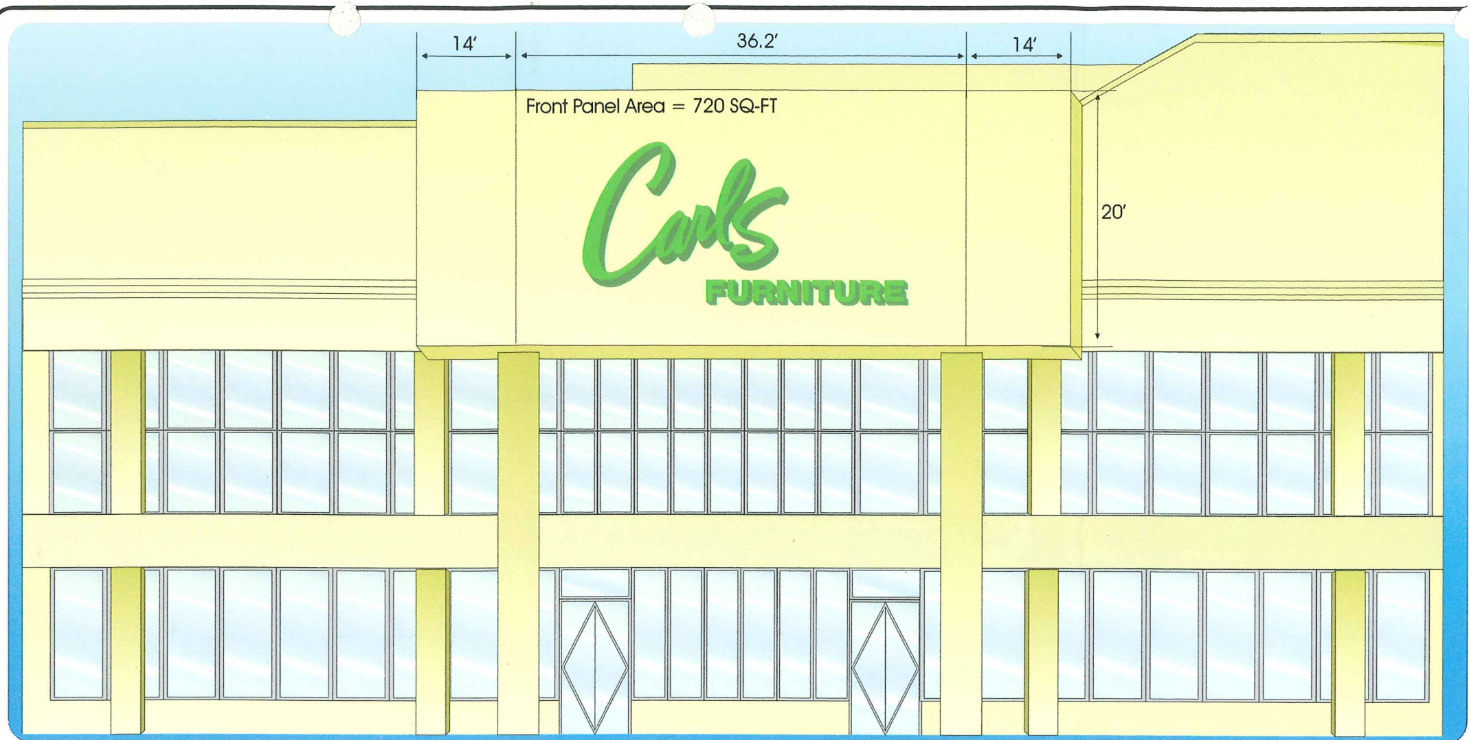
Set Illuminated Reverse Channel Letter. Scale-3/16" = 1' Sign Area = 300 SQ-FT
