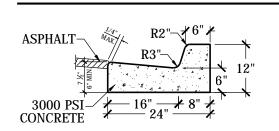
NOTE: WHEN USED ON HIGH SIDE OF ROADWAYS, THE CROSS SLOPE OF THE GUTTER SHALL MATCH THE SLOPE OF ADJACENT PAVEMENT AND THICKNESS OF THE LIP SHALL BE 6 INCHES.
