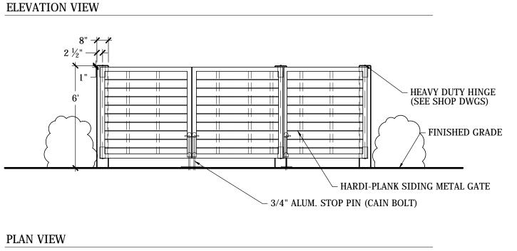
THE PLATE W/ 1" DIA. HOLES FOR STOP PINS TO LIMIT GATE CLOSING (DRILL PAVING 2" DEEP ALSO)
