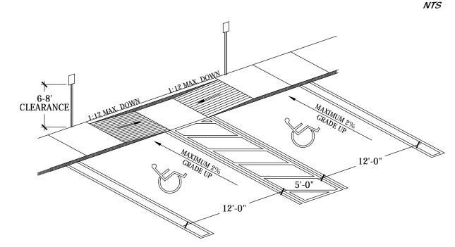
NOTE: IN THIS APPLICATION RAMPS CAN BE SEPARATED AND SIDEWALK CAN BE FLUSH ACROSS ALL HC SPACES
