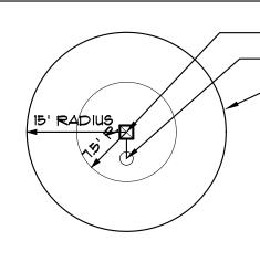
CONTRACTOR TO ADJUST ANY AND ALL TREES IN THE FIELD TO PROVIDE FOR MIN. 15' CLEARANCE FOR ANY SITUATIONS NOT PER PLAN. MINIMUM 7.5' CLEARANCE FROM ALL SMALL TREES
