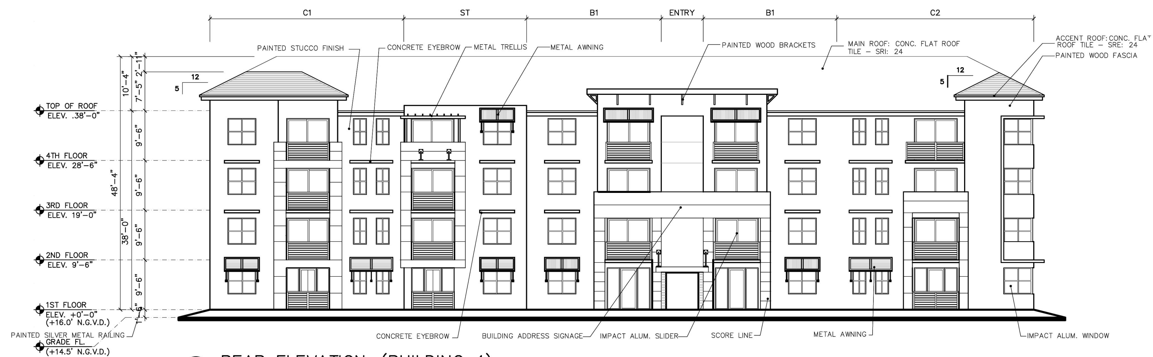
(B) REAR ELEVATION—(BUILDING 4) LAKE SIDE SCALE: 3/32"=1'-0"
