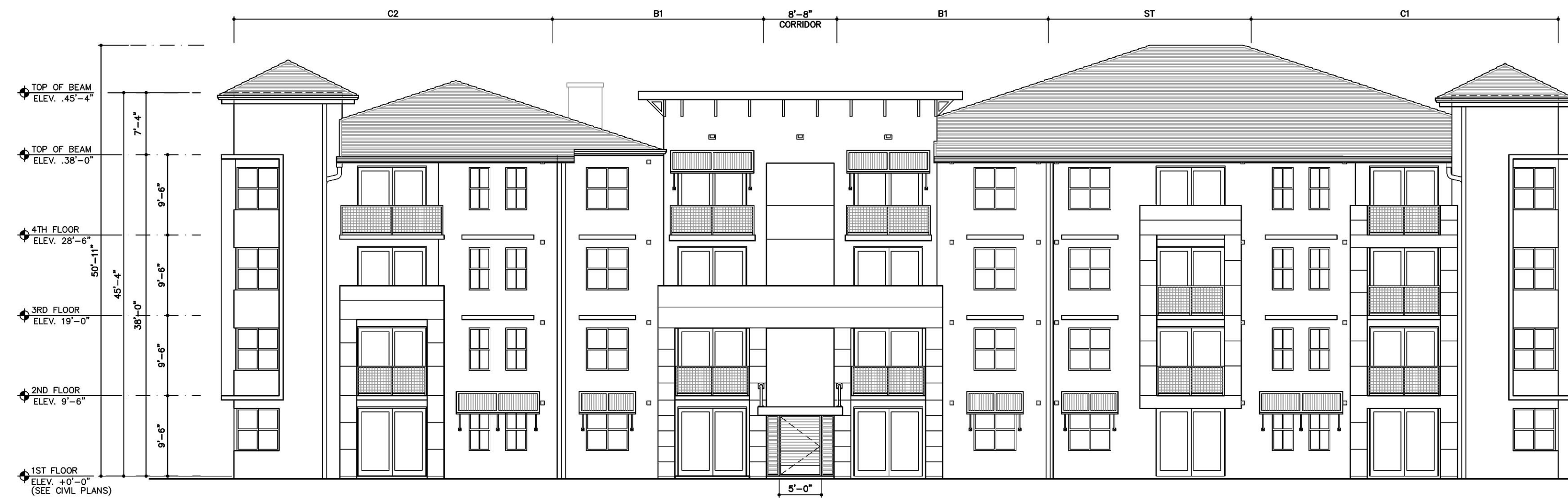
(B) REAR ELEVATION—(BUILDING 4) LAKE SIDE SCALE: 3/32"=1'-0"
