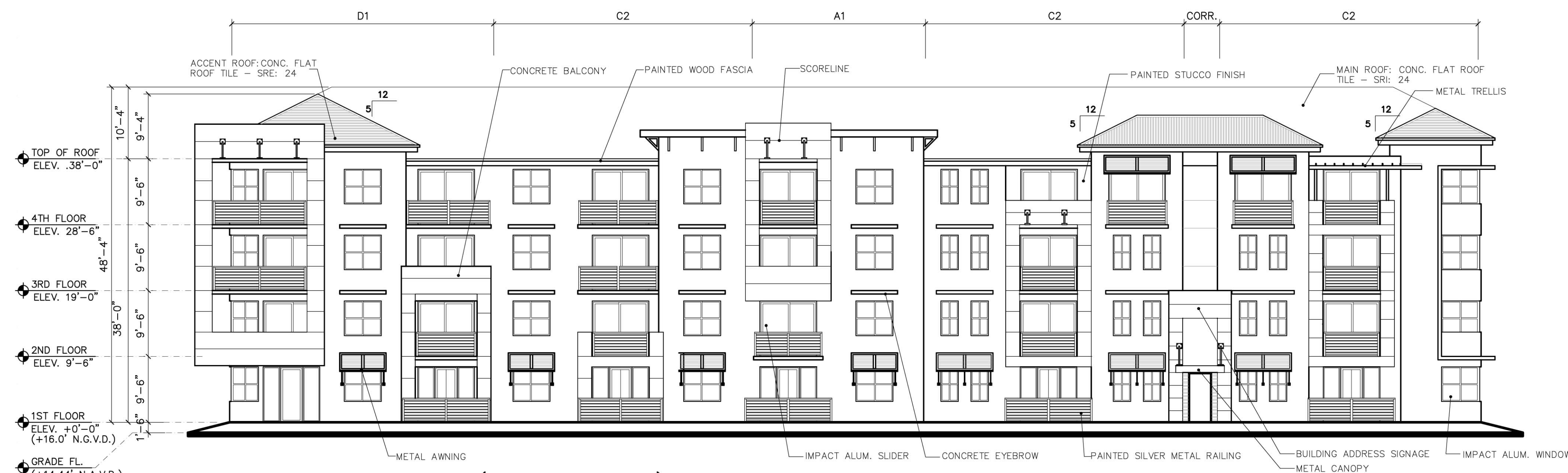
A FRONT ELEVATION - (BUILDINGS 5,6) INTERNAL SITE SCALE: 3/32"=1'-0"
