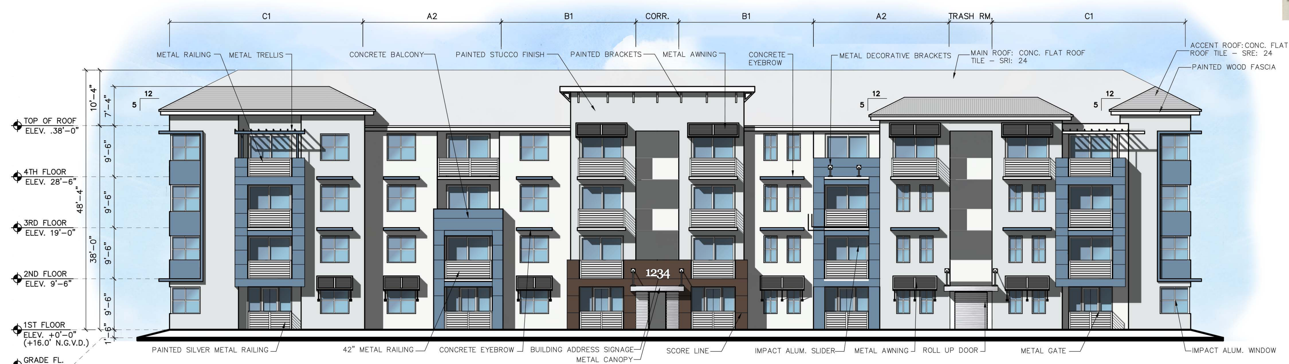
(B) REAR ELEVATION (BUILDING #1)
