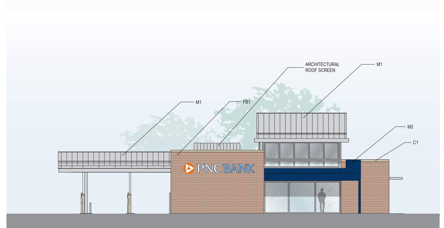
EXTERIOR BUILDING ELEVATION - FRONT SIDE
