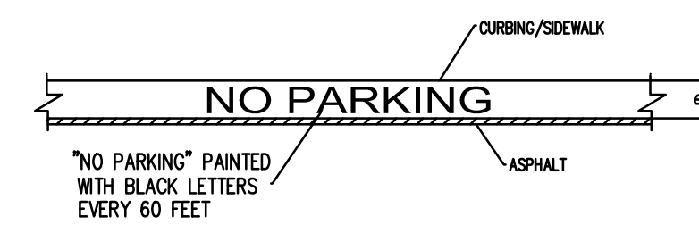
TYPICAL CURB MARKING AT CURB LOCATIONS
