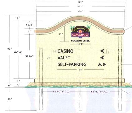
DeSign Stone wall sign system with (1) 76" x 116" x 12" body, (1) 6" x 120" x 16" base and (1) 25 7/8" x 120 " x 16" body topper
