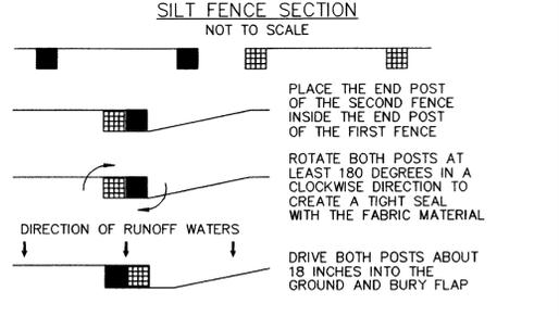
ATTACHING TWO SILT FENCES
