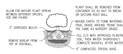
OR DISTURB ROOT BALL. -MOUND EARTH TO FORM WATERING SAUCER. FINAL GRADE AROUND TRUNK SHALL BE THE SAME AS NURSERY GRADE. FILL 2/3 WITH APPROVED PLANTING SOIL, THEN WATER THOROUGHLY. COMPLETE BACKFILL AFTER WATERING. " COMPACTED TOPSOIL BASE.
