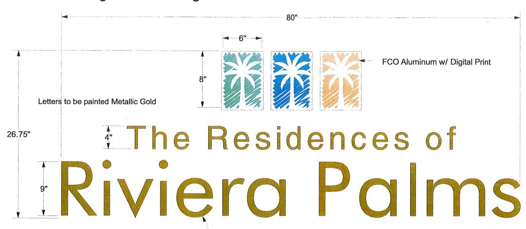
FLAT CUTOUT ALUMINUM LETTER STUD MOUNTED FLUSH TO CONCRETE WALL
