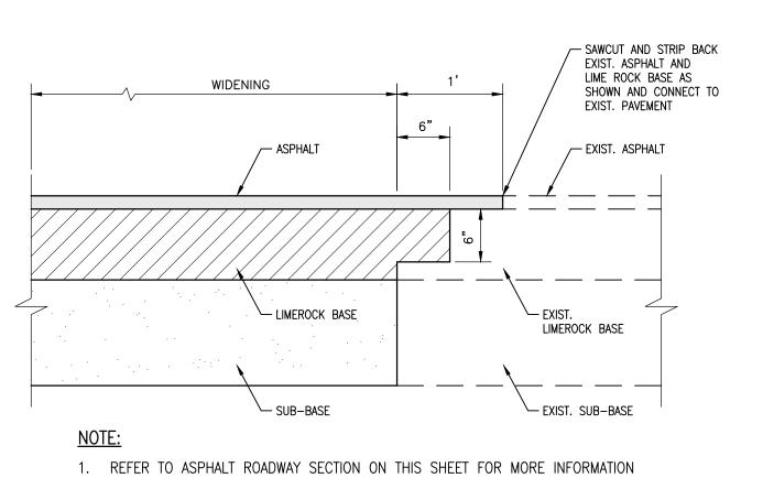
CONNECTION TO EXISTING PAVEMENT SCALE: N.T.S. CURRENT
